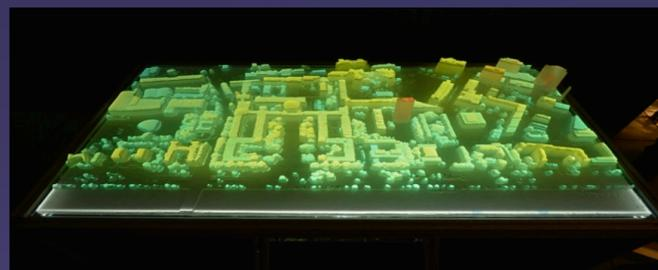
LuminoCity illuminated from projector base; display determined by measured height above ground level (data generated by LADAR).
